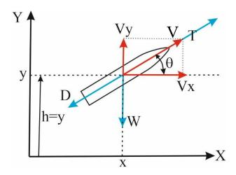
To simulate the rocket, integrate x, y,  $V_x$ ,  $V_y$  using the following equations:
